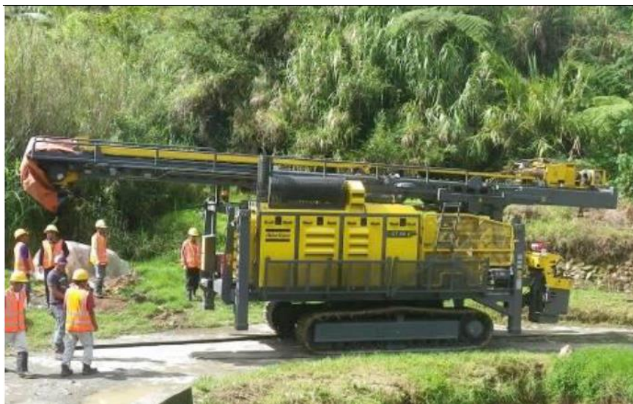
Figure 9_2 CT-20 Drill rig used to complete BRC60 (1,491m depth) for Gold Fields Philippines Holdings BV in 2013 (Source: IDM archives)
