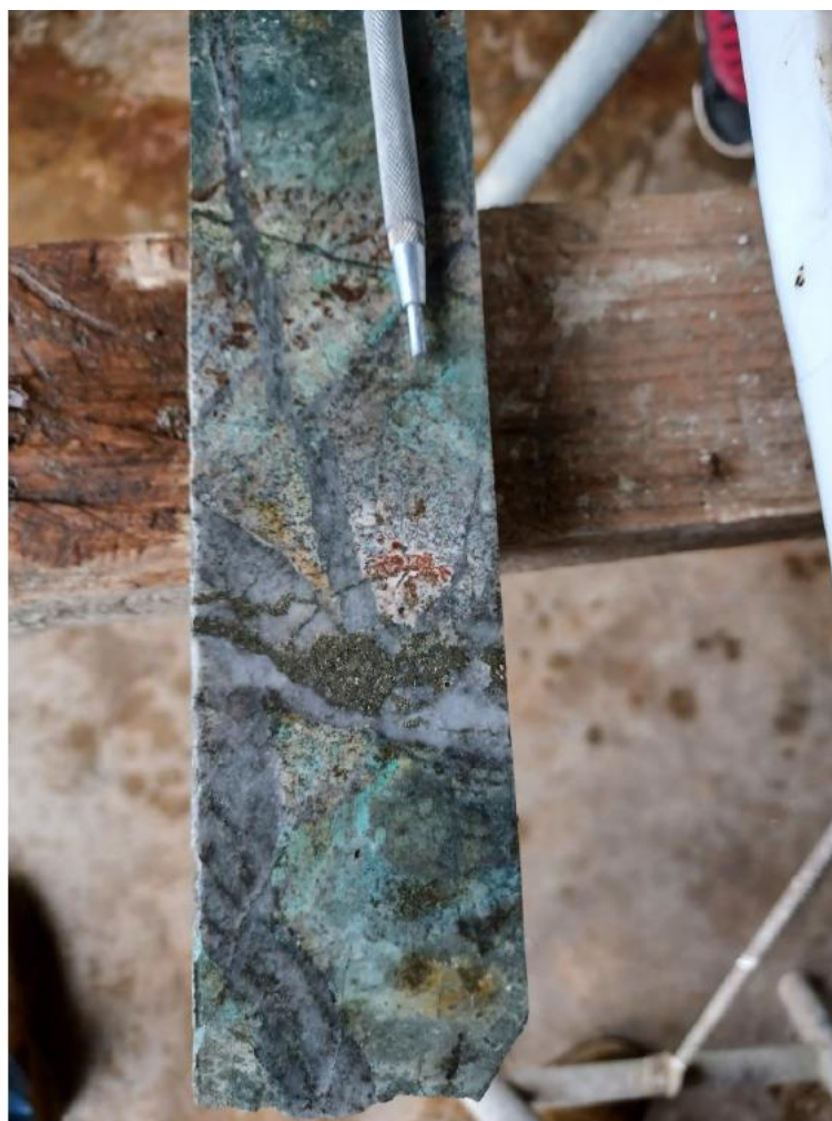
Figure 1.5_2 Mineralization in hole BRC60 from 851m to 854m averaging 1.06g/t Au and 0.78% Cu (Source Tuesley, 2021)
